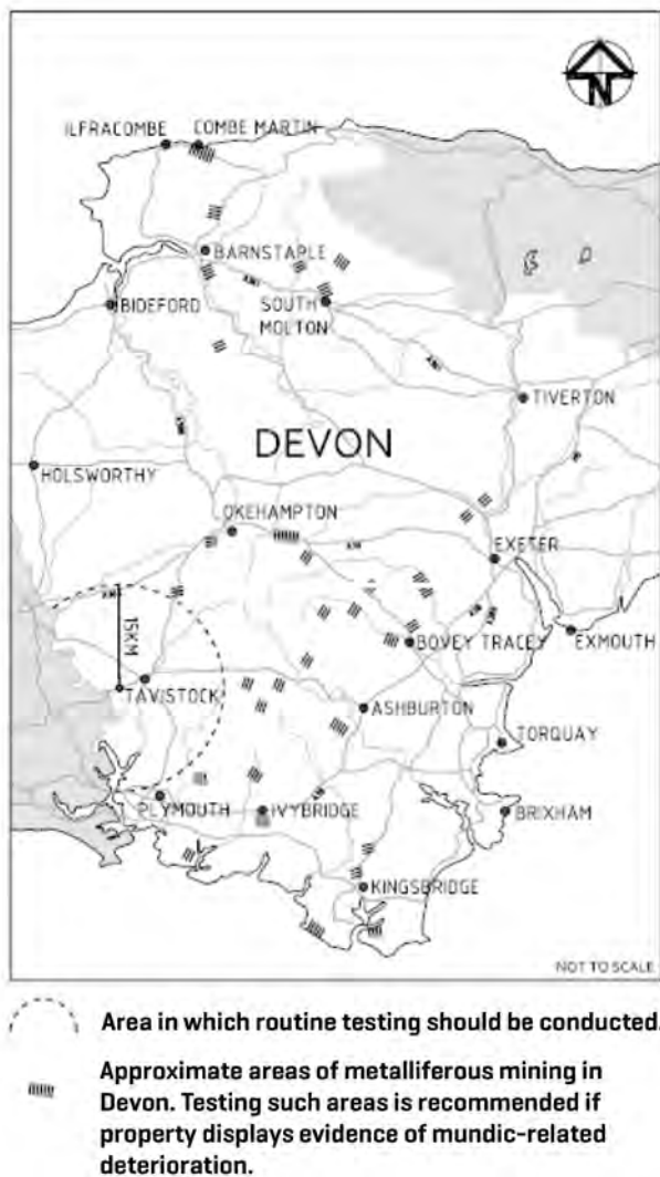
Figure 1: The dotted line on the map shows the approximate area of Devon where it is recommended routine testing be conducted. The dark bands indicate approximate areas of metalliferous mining in Devon; testing in and around such areas is recommended for properties displaying mundic-related deterioration
