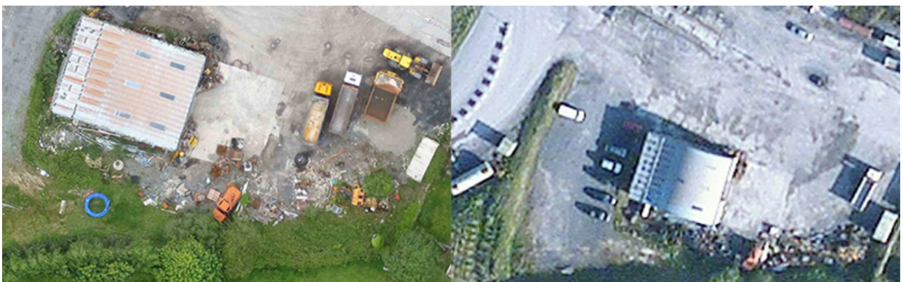
Figure 3: Drone imagery (centimetre resolution per pixel) versus satellite imagery (metre resolution per pixel)
